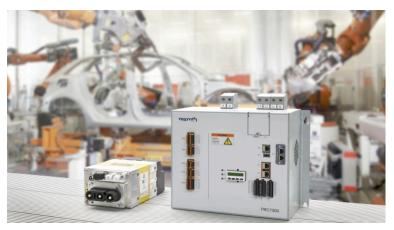
Industry 4.0-ready PRC7000 adaptive resistance welding controls feature a dual-processor architecture to enable high data transfer rates without affecting the welding process control.
