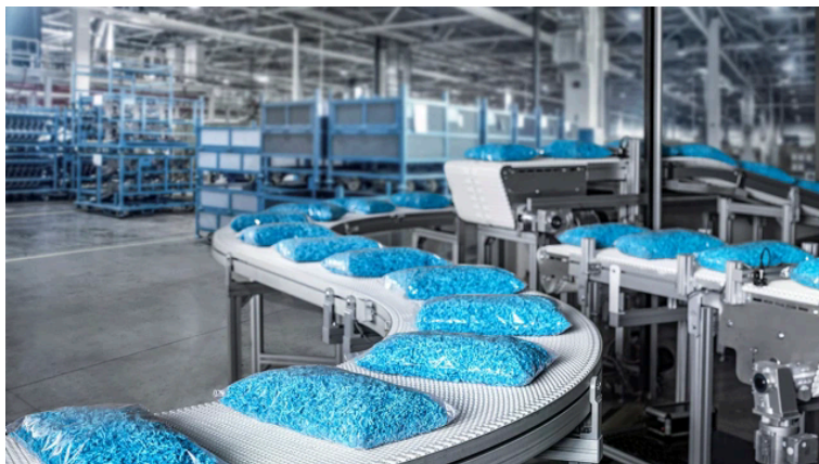
VarioFlow belt conveyor with a very fine-meshed, almost closed and flat surface for FMCG and pharmaceutical/healthcare applications
