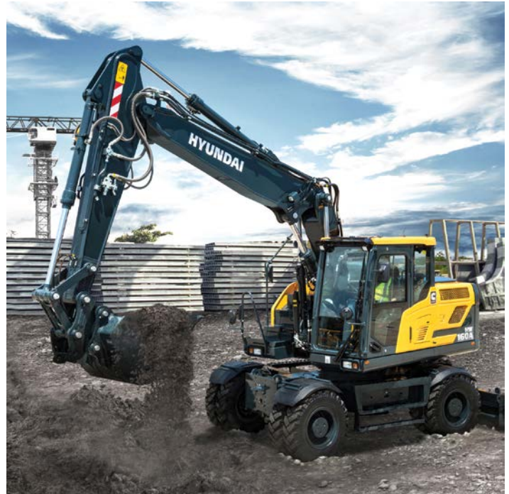
Excavators and wheeled loaders have different functions, but with the RS modules from Bosch Rexroth they have a uniform valve platform for the working hydraulics – including the option of electronic control (photo: Hyundai Construction Equipment).
