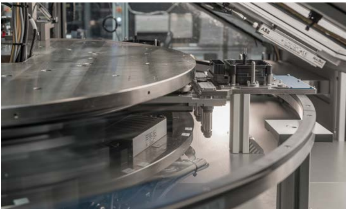
Bosch Rexroth's Flexible Transport System (FTS) is a specially developed linear motor transport unit suitable for easy integration into the Rexroth TS 2plus conveyor. A main benefit is that the FTS features omnidirectional transport where every carrier's movement – direction, speed, start and stop rates – can be individually programmed.
