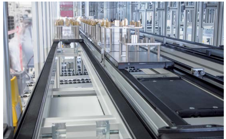
A key section on the new line uses the Rexroth TS 2plus pallet conveyor (like the one shown here), a robust, versatile and highly modular setup that can carry loads up to 240 kilograms. It supports transport speeds up to three meters per second and features a complete series of pallet-based transfer, positioning and control components.
