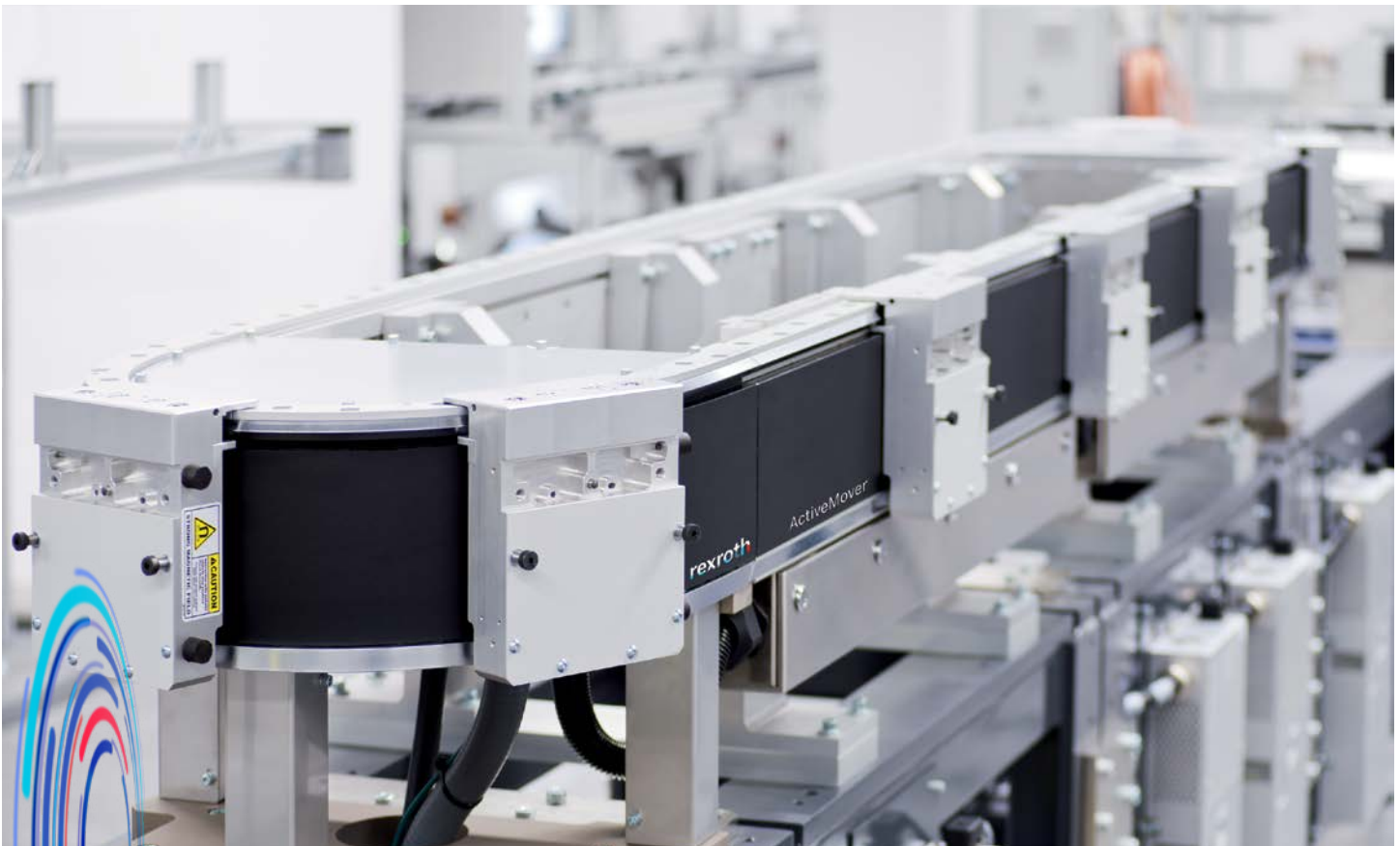
Linear transfer systems like Bosch Rexroth's ActiveMover offer food packaging lines extremely fast transport with precise positioning that can be easily adjusted with simple programming.
