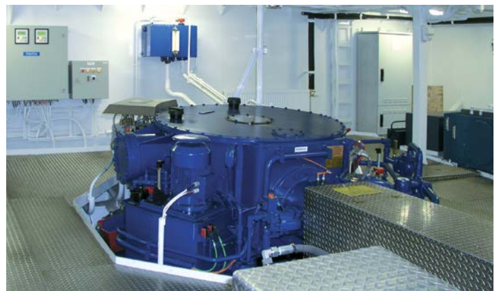
▲ Maximum maneuverability in tight spaces made possible by the cycloidal drive – equipped with Rexroth drive technology
