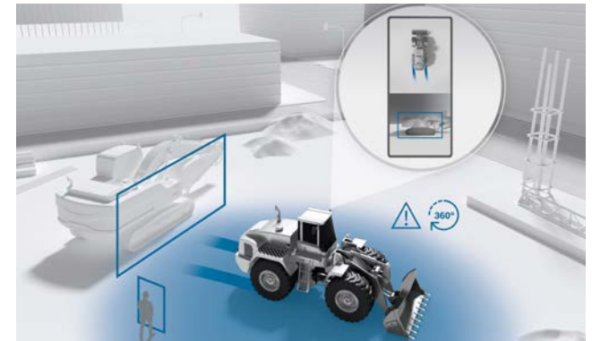
Multi-camera system provides 360° surround view and virtual camera movement depending on the steering angle.
