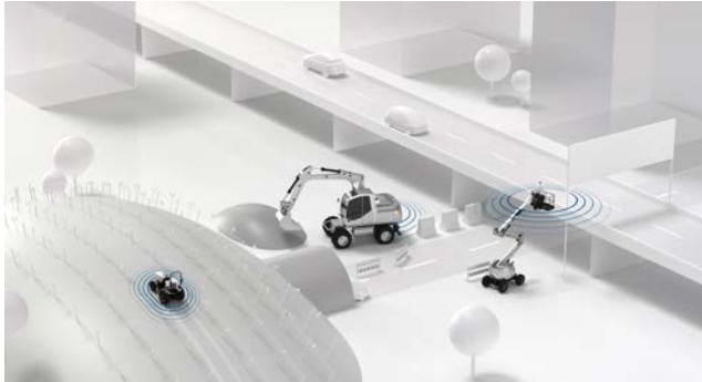
Specific examples for ultrasonic sensors are the man basket or the blind side of the excavator.
