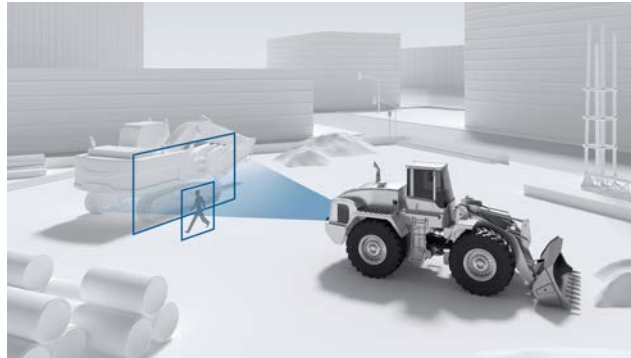
In addition, the radar sensor enables object tracking for the assumption of object movements.
