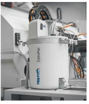
The compact CytroPac hydraulic power unit is a revolutionary solution for machine tool design. With every HPU function packaged into one unit including a Sytronix variable-speed pump drive, i4.0-enabled interface, and a no-hassle cooling and degassing tank design, the plug-and-play CytroPac can help you achieve new levels of productivity.
