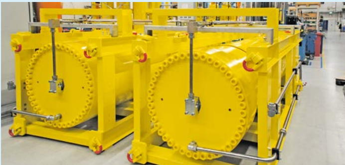
◀ Xayaburi accumulator unit, Laos 2 x 1,850 l hydraulic medium, 7 x 1,250 l N 2
