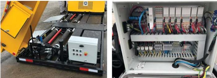
Vehicles drive on top of the VIS-Check, with the machine applying force to each wheel, which the vehicle must counter by applying the brakes. At the end of a test, the VIS-Check produces a final report on the health of a vehicle's brakes, providing a pass/fail grade. In addition to making sure the brakes comply with DOT specifications and CVSA guidelines, the unit is able to find otherwise undetectable issues in need of repair, enhancing vehicles' overall safety on the road.
