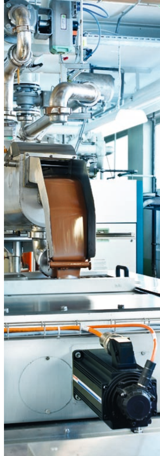
Molding equipment for bar chocolate
