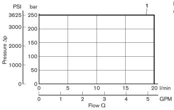
Measured with the solenoids at their operating temperature, 10% under voltage and without pre-loading of the tank.
