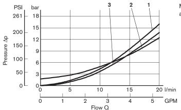
Measured with hydraulic fluid ISO-VG32 at  $45^{\circ} \pm 5^{\circ}$  C (113°  $\pm$  9° F); ambient temperature 20° C (68° F).
