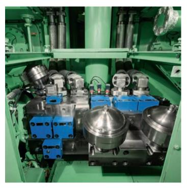
Large 2-stroke engines have engine oil (additive enriched) that is injected into special delivery chambers via the cylinder liner, at a rate dependent upon engine load. The piston rings ride on this film of lubricant. Manufacturers have developed a variety of similar lubrication systems. They all inject the oil under pressure and ensure that it is evenly distributed along the cylinder liner. The time window for the injection process is 4 to 20 msec.
