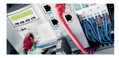
The control translates parameter changes into commands for the drive axes in real time. The special characteristics of hydraulic control such as closed-loop controls of state, position, pressure/force, and velocity as well as synchronization controls are stored in algorithms, thus simplifying automation.
