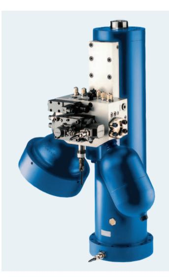
▲ Compact: the function unit consisting of servo control block and servovalve as well as diaphragm-type accumulator is fitted directly on the hydraulic cylinder
