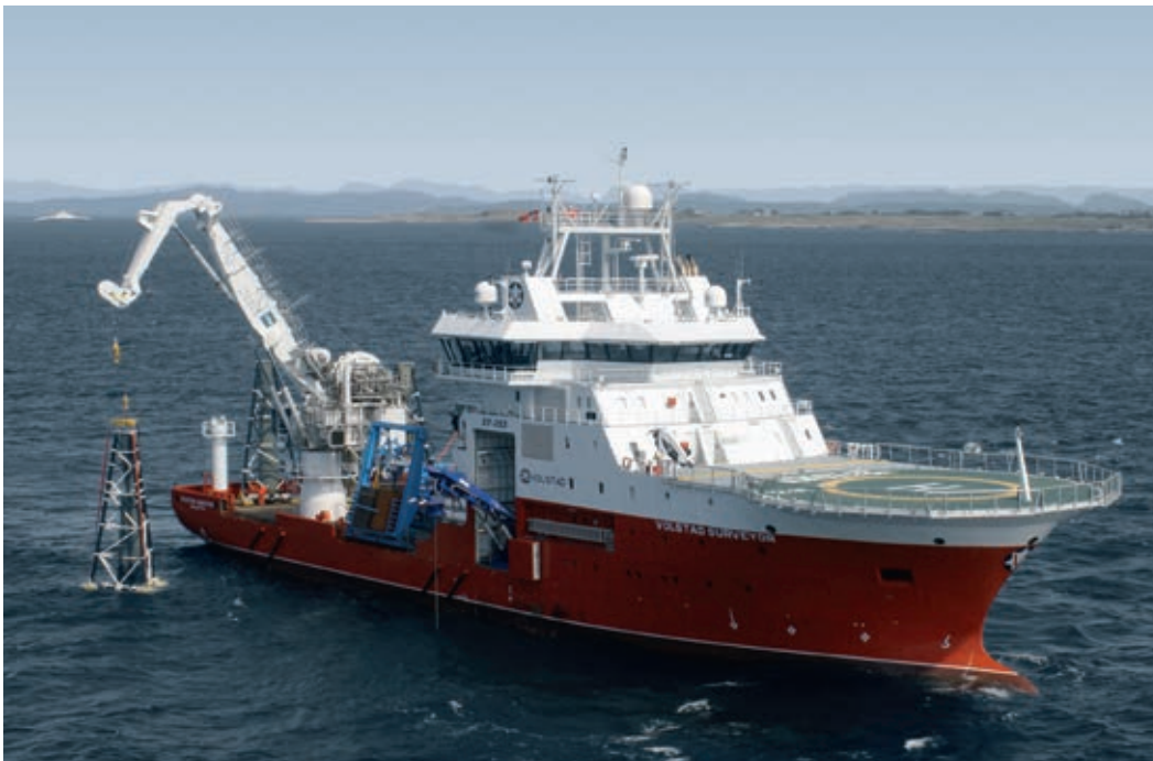
◀ Offshore knuckle boom crane with active heave compensation
