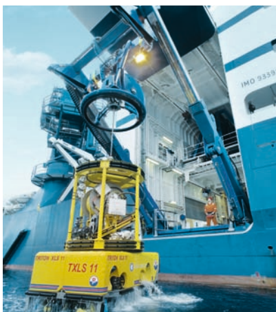
Launch And Recovery System (LARS) from ODIM, Photo: Tony Hall
