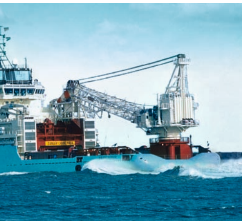
160-ton crane for multi-purpose vessel from KENZ-FIGEE
