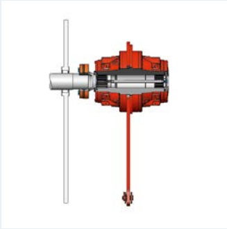
▲ Torque arm mounted motor with shaft coupling.
