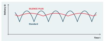
The flow pulsation lowered by 75% reduces vibration in the machine, and a 35% lower frequency produces a more pleasant sound.
