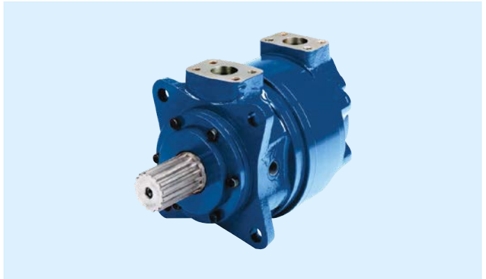
▲ MV057 – 500 rpm, 3016 lb-ft (4089 Nm) Offered in A [3000 psi (207 bar)] or D version [4500 psi (310 bar)]. The same features offered in the 37 Series are available in a motor that's one inch longer. Modified SAE D mount.
