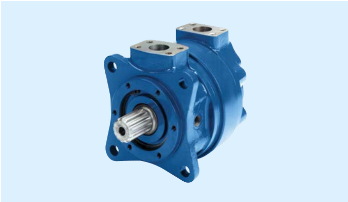
▲ MV037 – 1000 rpm, 2007 lb-ft (2721 Nm) Offered in A [3000 psi (207 bar)] or D version [4500 psi (310 bar)]. Splined, tapered, straight keyed, and double output shafts are standard, along with through holes to 1 1/2". Optional thrust and radial load bearings with substantial capacity, tach pickups, double stacks (up to twice the torque), and brake mounts available. SAE D mount.
