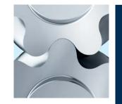
Continuous tooth contact reduces operating noise: A non-involute rounded tooth profile, combined with helical cut teeth, forms the heart of the SILENCE PLUS. Thanks to permanent tooth contact the fluid is transported almost continuously and noiselessly. The possibility of noise from trapped oil between the tooth flanks is prevented in the first place.
