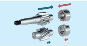
▲ Hydrostatic bearing ensures long service life: The high performance and long service life of the SILENCE PLUS is due to a Rexroth patented solution: Hydrostatic grooves provide wearfree compensation for the internal axial forces generated in the helical gear – even at pressures up to 280 bar!
