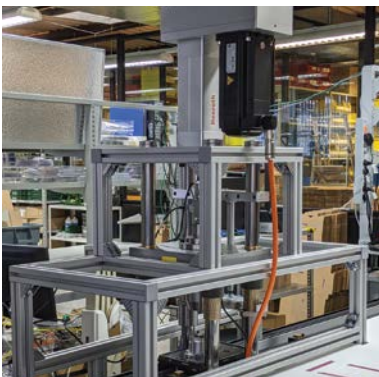
Production of different types of rotary encoders at Sensata: the Smart Function Kit for pressing tasks reduces engineering, commissioning, and quality assurance costs. (Copyright: Sensata)
