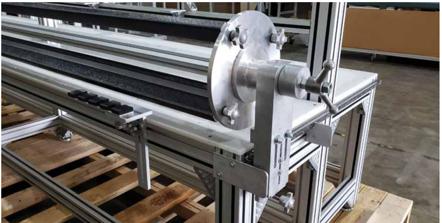
■ A carousel-style fixture not only improved productivity, it also reduced floor space and improved part flow.
