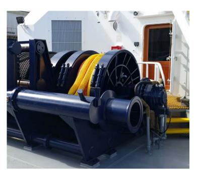
In a geared system, Durar says, a single revolution of the drum could translate into 1000 revolutions by the time the last gear is reached. But in a direct drive system, one turn of the drum is just one turn of the Hägglunds motor, which is further protected by its low moment of inertia. "I've got to put something out there that customers can beat the hell out of," says Durar. "At the end of the day, Hägglunds motors can take a beating."
