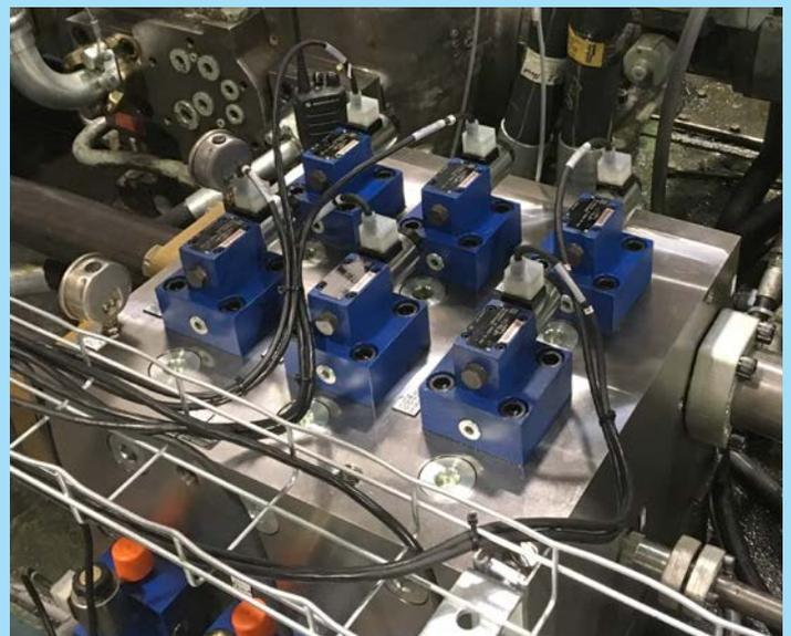
Leak-prone, obsolete legacy spool valves (left) were replaced with a custom manifold system supplied by Bosch Rexroth (right). The new manifold system helps reduce dead cycle time by three seconds, as well as reducing system shock and hydraulic fluid leakage.
