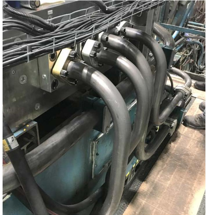
Part of the upgrade included replacing a tangle of welded piping with a simpler arrangement of weldless steel piping, another step taken to eliminate potential points of fluid leakage.
