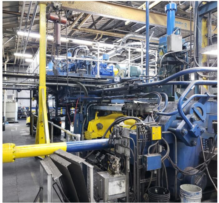
**The Bosch Rexroth team worked closely with Superior Extrusion to design a drop-in solution comprised of Rexroth A4VSO 500 axial piston pump, custom manifold, Rexroth LC and LFA logic valves and custom-programmed HACD digital electronic control.**
