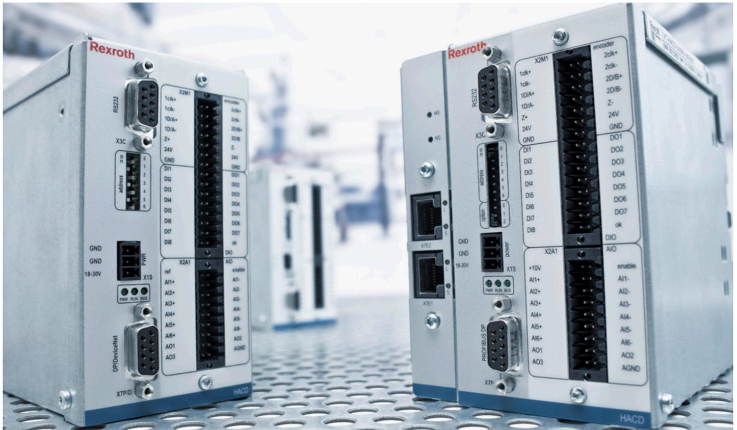
**An HADC digital electronic control was configured to take the existing analog signals that previously controlled the legacy pumps and use those outputs to control both the A4VSO piston pump and the LC and LFA valves.**
