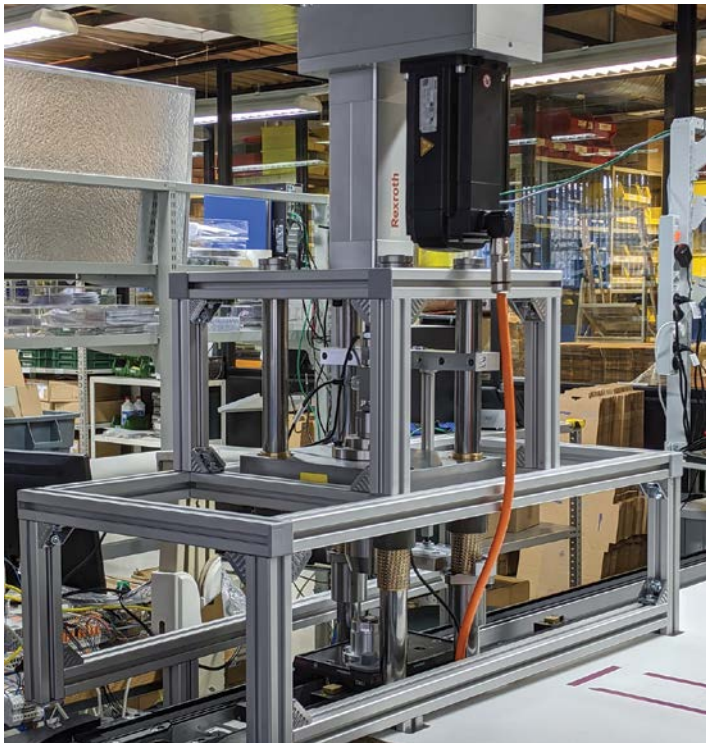
Fig. 4: Production of different types of rotary encoders at Sensata: the Smart Function Kit for pressing tasks reduces engineering, commissioning and quality assurance costs. (Copyright: Sensata)
