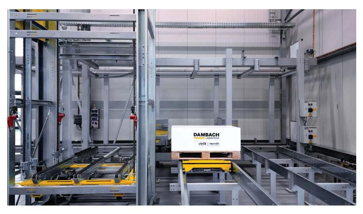
The shuttle runs completely independently with its own power supply. This is provided via PowerCaps for energy storage purposes. As a result, the system can run independently of the storage and retrieval machine in the warehouse channels and store and retrieve goods. The PowerCaps can be recharged in just a few seconds on the storage and retrieval machine or transport vehicle, which means that the system can operate 24/7 without interruptions.
