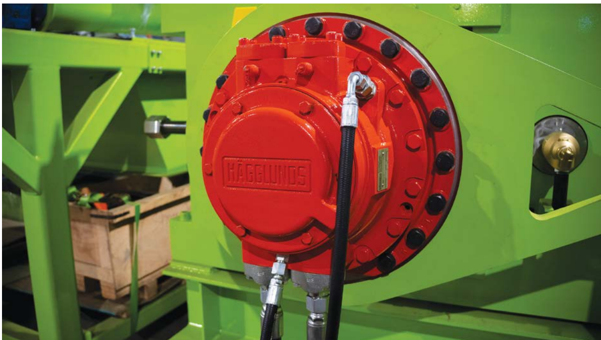
The direct drive hydraulic motor delivers the full energy of operation to the shaft being driven and uses the hydraulic fluid as the medium to absorb the surges and drops, rather than having mechanical gears that lash in a gearbox system.
