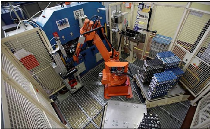
Fig. 9: Cartridge valves automated production lines
