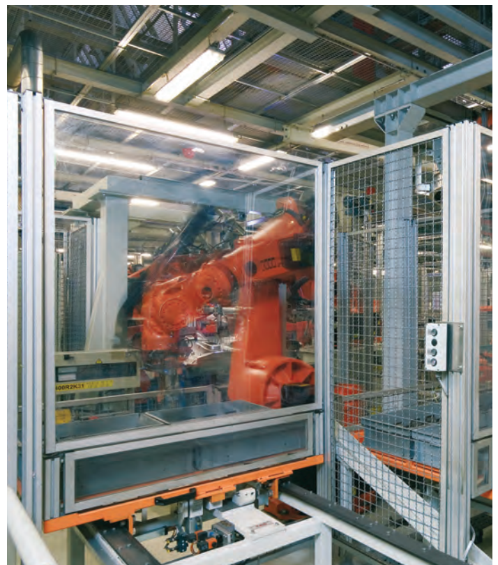
Custom safety structures with corrosion-protected surfaces protect workers and equipment from workplace accidents.
