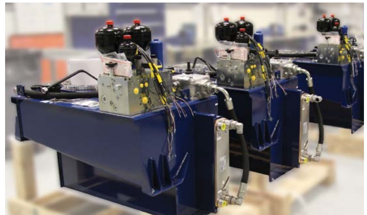
Hydraulic power units designed for use in a serial application can incorporate unique or specific features for the machine series.
