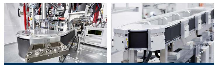
Bosch Rexroth's ActiveMover is a highly dynamic, flexible transfer system based on linear motors. ActiveMover unlocks the potential to increase productivity for small batch sizes, thanks to its quick and precise positioning of workpiece pallets.
