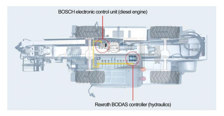
Innovative new solutions at work that elevate the connectivity with machines—the way information is exchanged between diesel control and hydraulics control, for example.
