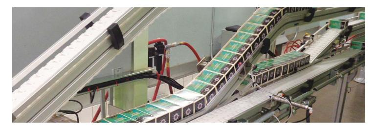
Modern tea bag production with the flexible conveyor system VarioFlow *plus* from Rexroth
