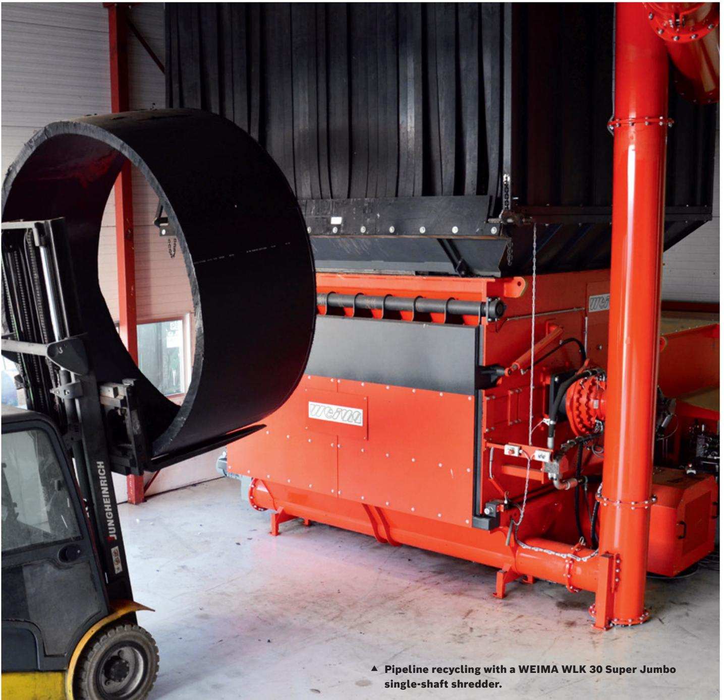
▲ Pipeline recycling with a WEIMA WLK 30 Super Jumbo single-shaft shredder.
