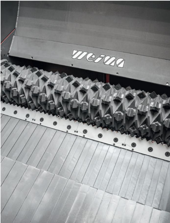
▲ WEIMA V rotor, equipped with cutting knives.
