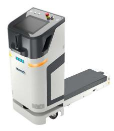
Touchscreen and 3D obstacle detection: the new ActiveShuttle with Advanced Interaction transports small load carriers autonomously, safely and with a high degree of flexibility. (Image source: Bosch Rexroth AG)
