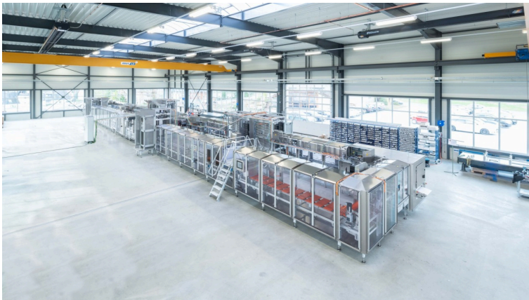
Tidy and easily accessible: The modular ConfecPRO with decentralized drive technology from Bosch Rexroth. (Image source: WDS)
