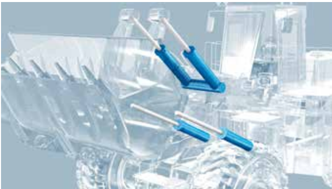
Use of hydraulic cylinders in a wheel loader
