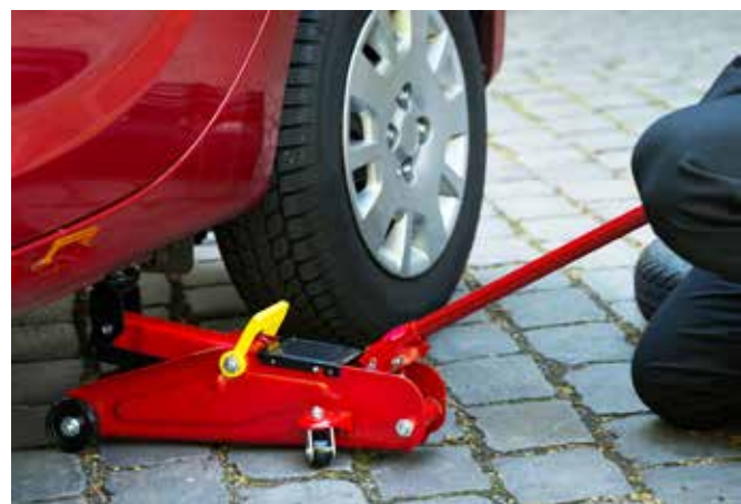
Hydraulic jack (practical example of application of force and path transmission)
